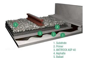
The membrane is pre-heated before being applied and then the primed substrate and the bituminous sheet are heated alternately. The welding is performed: either manually with a flame, or automatically using hot air (MACADEN system).
