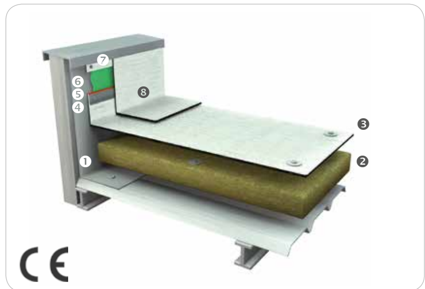
① Free standing metal upstand fixed on the steel deck ② Thermal insulation panels ③ FLAGON® EP/PR membrane ④ Pre-drilled metal bar: FLAGORAIL ⑤ FLAGOFIL cord ⑥ FLEXOCOL bonding adhesive ⑦ Mechanically fastened colaminated strip ⑧ FLAGON® EP/PR for upstand
