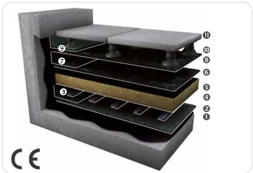
① Primer ② Vapour barrier ③ Vapour barrier corner reinforcement ④ SOPRACOLLE 300 N ⑤ Thermal insulation panel ⑥ 1 st waterproofing layer SOPRALENE® FLAM 180 ⑦ Corner reinforcement SOPRALENE® ⑧ 2 nd waterproofing layer SOPRALENE® FLAM 180 AR ⑨ 2 nd layer for upstand SOPRALENE® ⑩ SOPREMA support pads ⑪ Paving slabs
