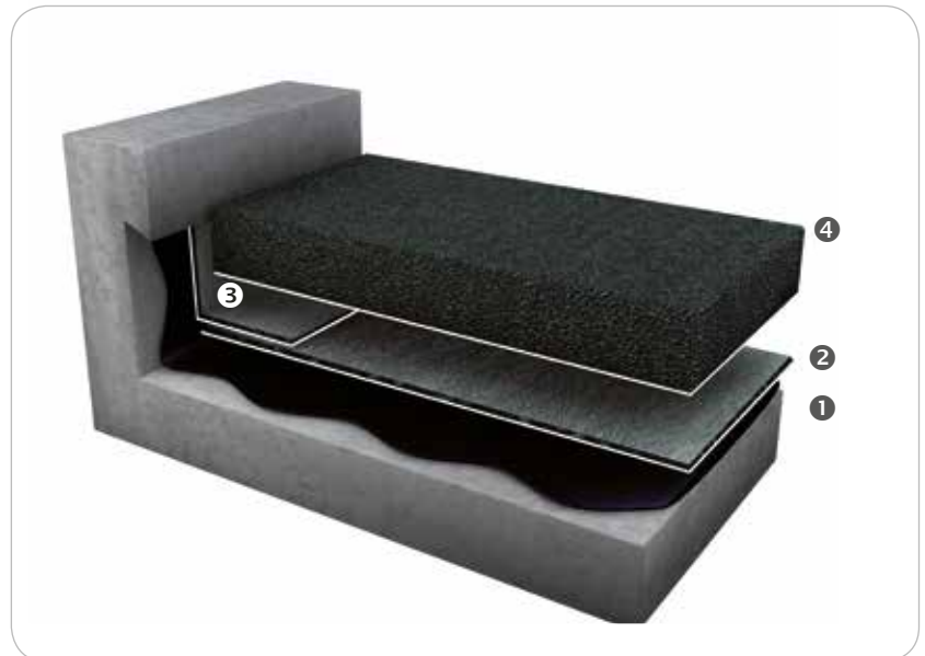
① Primer ELASTOCOL® 500 ② SOPRALENE® FLAM ANTIROCK® P ③ Corner reinforcement SOPRALENE® FLAM ANTIROCK® P ④ Hot-rolled asphalt
