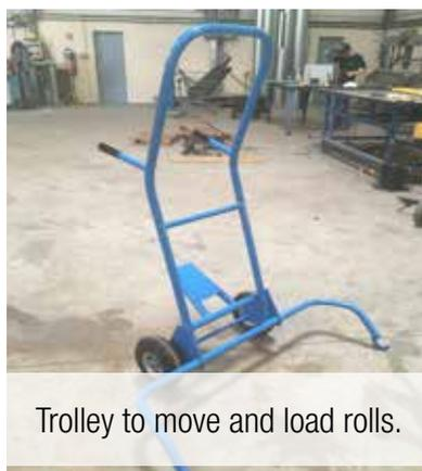
Trolley to move and load rolls.
