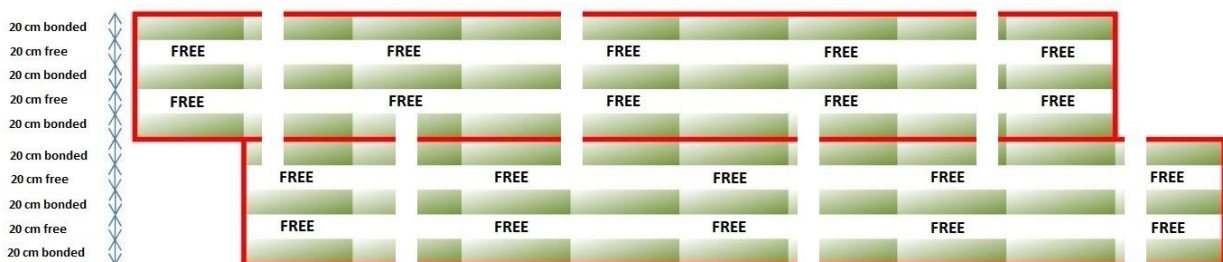
Double gluing application with 350 g/m 2 - 175 g/m 2 on each side - Pressing carefully
