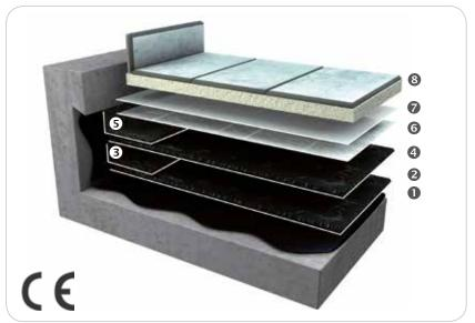
● Primer ② 1st waterproofing layer ELASTOPHENE® FLAM 25 ⑤ Corner reinforcement SOPRALENE® ⑤ 2st waterproofing layer SOPRALENE® FLAM 180 AR ⑤ 2st layer for upstand SOPRALENE® FLAM S 180-35 ⑥ NTS 170 separating sheet ⑥ PE Foil (100μ) ⑥ Sopped with titles
