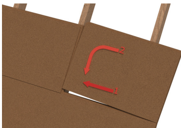
Fix ensuring that the tongue is fully engaged by locating end tongue first then slide down onto the lower board.
